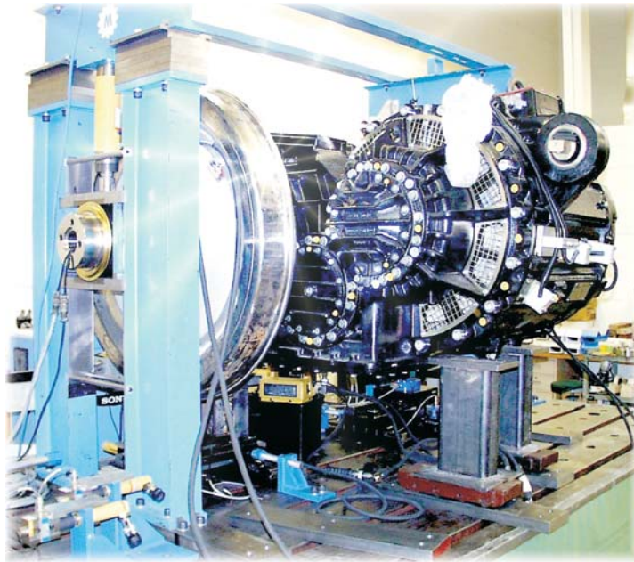
Calibration of Instrumented wheelsets with gearbox and traction motor attached.
