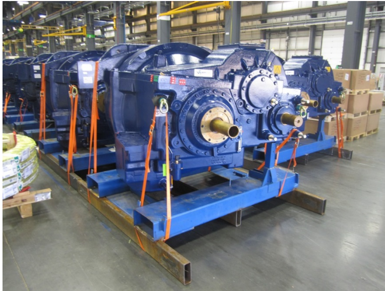
Photo 1: Gearbox mounted on transport sled and secured with 4 - 1 ½ in. polyester straps
