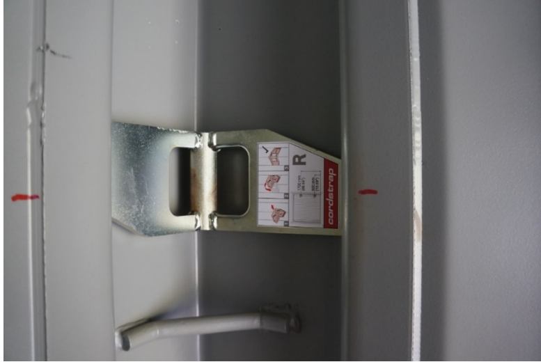
Photo No. 1: CornerLash® strap anchor installed
