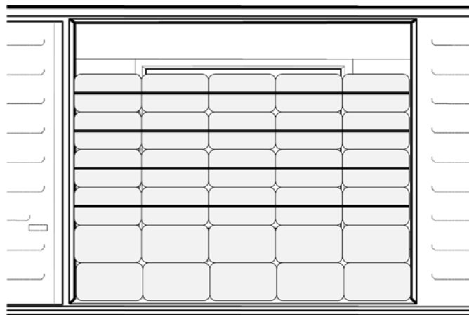
Figure No. 7 – Doorway protection for individual bales (wood pulp) in single plug door boxcars
