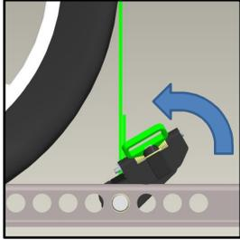
**2.** Insert Mandrel of Anchor Restraint completely through both holes of the chock track (to right side of wheel) as shown. See **NOTE** for strap orientation.
