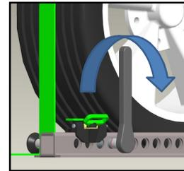
**4.** Pull strap taut over top of tire and insert cleats into tread keeping the strap centered on the tire. Remove any twists keeping the strap flat with printed text facing up.
