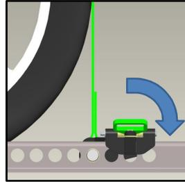
**3.** Rotate the Retainer Plate down until the spring loaded Lock Lever snaps into adjacent chock track hole.
