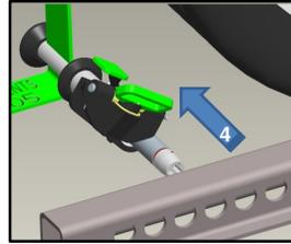
**3.** Rotate Retainer Plate up to clear track.
