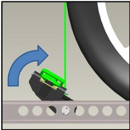
**5.** Insert Mandrel of Ratchet Restraint completely through both holes of the chock track (to left side of wheel) as shown. See **NOTE** for strap orientation.
