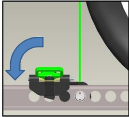
**6.** Rotate the Retainer Plate down until the spring loaded Lock Lever snaps into adjacent chock track hole.
