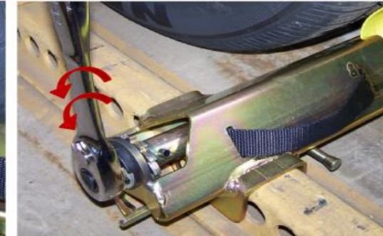
Push the Release Pawl Lever down with your foot to release the strap.
