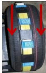
A) The strap is centered in the middle of the tire.
