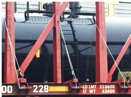
Examples photos of properly secured centerbeam cables
