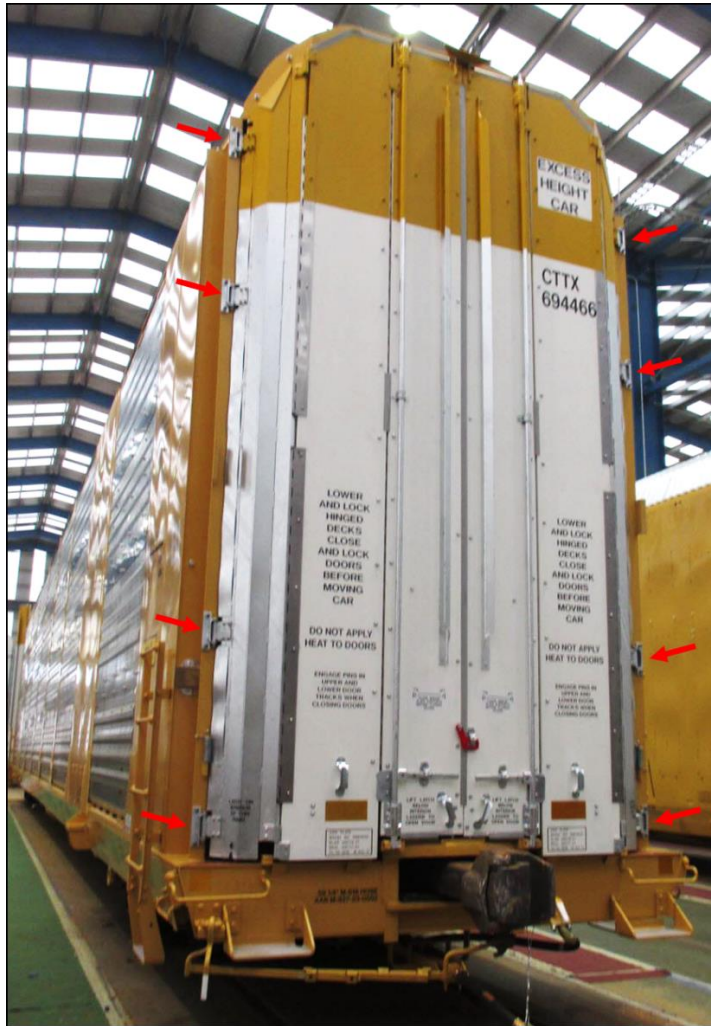
Each corner of the car has four hinges supporting the end doors
