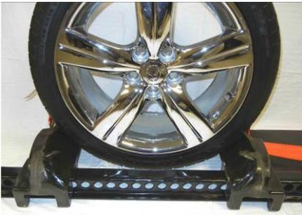
Place the chock pair on either side of the automobile tire with the winch mechanism away from the automobile body.
