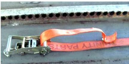
A photograph showing the orange strap fully unwound from the winch mechanism, lying flat on a metal surface.                       | <p>When the over-wound strap is unwound the strap should be free in the winch with nylon nut and bolt retainer.<br/>Lubricate the winch before putting it back into service. Refer to the Maintenance section.</p>                                                         |
