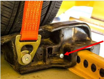
On the inside chock (the chock toward the center of the automobile, with only the strap latch), pull the pawl back to retract the locking pin and lift the pawl up to restrain the pin against the spring force.
