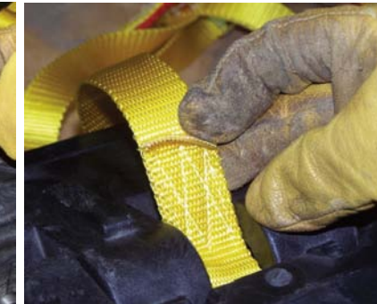
4) Assure that Cleats are correct to engage tire tread - seam facing up.
