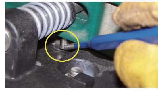
2) It may be necessary to center Roll Pin to thru-hole in Articulation (as shown).
