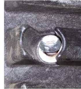
3) Insert Carriage Bolt Replace and start Nut (assure washer is present)
