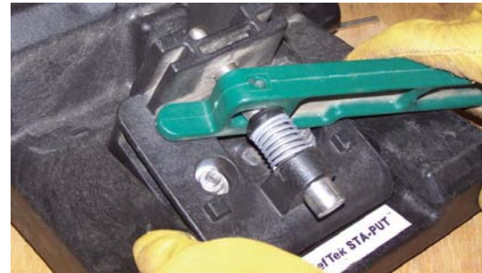
3) Pull Back on Release Lever disengaging Latching Pin. (May have to pry back if broken too close to Pin)
