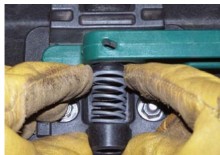
5) Replace Release Lever and re-position Spring and Follower Ball.
